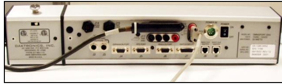
Figure 29: Lane Data and Horn Start Plugs
