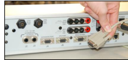
Figure 31: Serial Cable Connection to Console
