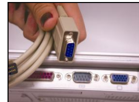
Figure 32: Serial Cable Connection to Computer
