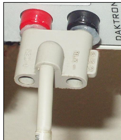
Figure 8: Insert GND Side to Black Female Jack
