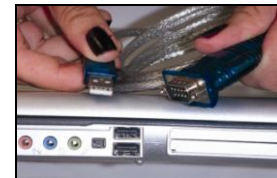
Figure 33: Using a USB to Serial Adaptor
