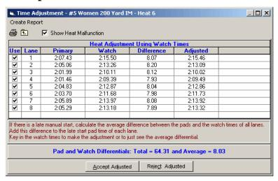
In this example, there was a late manual start of the electronic timing system and the times from the pads are equally incorrect for all the lanes in the heat. The order of finish and the absolute difference of the times between the swimmers are believed to be accurate.
